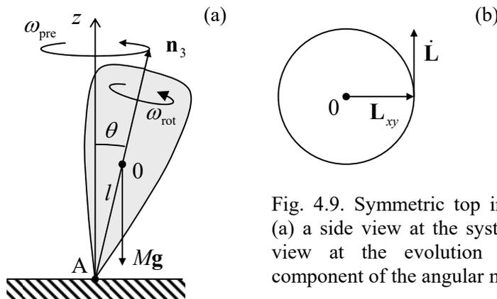
Fig. 4.9. Symmetric top in the gravity field: (a) a side view at the system and (b) the top view at the evolution of the horizontal component of the angular momentum vector.
