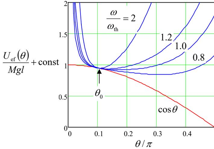
Fig. 4.11. The effective potential energy  $U_{\text{ef}}$  of the symmetric top, given by Eq. (82), as a function of the polar angle  $\theta$ , for a particular value (0.95) of the ratio  $r \equiv L_z/L_3$  (so that at  $\omega_{\text{rot}} \gg \omega_{\text{th}}$ ,  $\theta_0 = \cos^{-1}r \approx 0.1011\pi$ ), and several values of the ratio  $\omega_{\text{rot}}/\omega_{\text{th}}$  – see Eq. (85).
