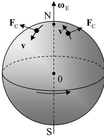
Fig. 4.16. Coriolis forces due to the Earth's rotation, in the Northern hemisphere.
