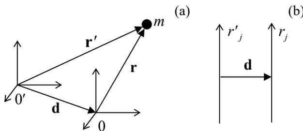
Fig. 4.4. (a) A general coordinate frame’s shift from the center of mass, and (b) a shift perpendicular to one of the principal axes.
