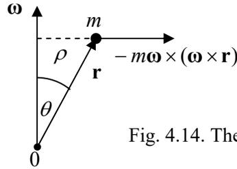
Fig. 4.14. The centrifugal force.
