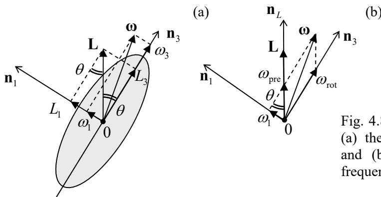
Fig. 4.8. Free rotation of a symmetric top: (a) the general configuration of vectors, and (b) calculating the free precession frequency.
