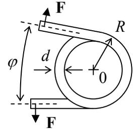
7.16. Use Eqs. (99) and (100) to recast Eq. (101b) for the torsional rigidity  $C$  of a thin rod into the form given by Eq. (101c).
