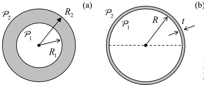
Fig. 7.7. The spherical shell problem: (a) the general case, and (b) the thin shell limit.
