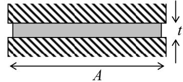
7.3. Two opposite edges of a thin but wide sheet of an isotropic elastic material are clamped in two rigid, plane, parallel walls that are pulled apart with force  $F$ , along the sheet’s length  $l$ . Find the relative extension  $\Delta l/l$  of the sheet in the direction of the force and its relative compression  $\Delta t/t$  in the perpendicular direction, and compare the results with Eqs. (45)-(46) for the tensile stress and with the solution of the previous problem.
