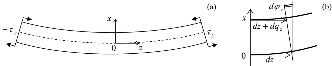
Fig. 7.8. Rod bending, in a local reference frame (specific for each cross-section). The bold arrows show the simplest way to create the two opposite torques  $\tau_y$ : a couple of opposite forces for each torque.
