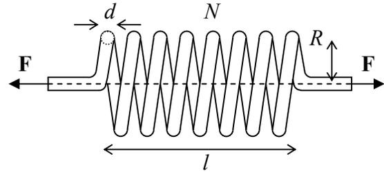
7.15. The coil studied in the previous problem is now used as what is sometimes called the *torsion spring* – see the figure on the right. Find the corresponding spring constant  $d\tau/d\phi$ , where  $\tau$  is the torque of the external forces  $\mathbf{F}$  relative to the center of the coil (point 0).
