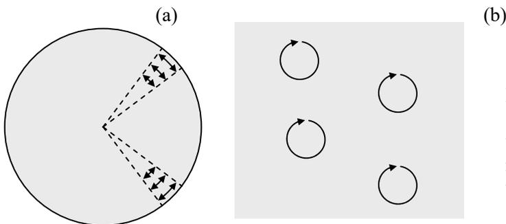
Fig. 7.14. Particle trajectories in two different transverse waves with the same velocity: (a) torsional waves in a thin round rod and (b) circularly polarized waves in an infinite (or very broad) sample.
