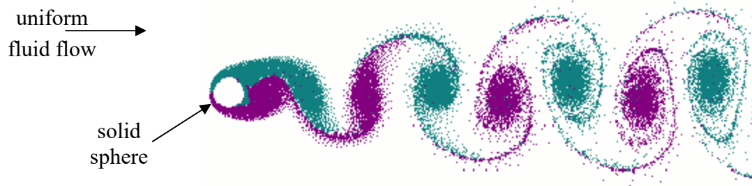
Fig. 8.16. A snapshot of the turbulent tail ( wake ) behind a sphere moving in a fluid with a high Reynolds number, showing the so-called von Kármán vortex street . Adapted from the original (actually, a very nice animation, http://www.mcef.ep.usp.br/staff/jmeneg/cesareo/vort2.gif ) by Cesareo de La Rosa Siqueira, as a copyright-free material, available at https://commons.wikimedia.org/w/index.php?curid=87351 .
